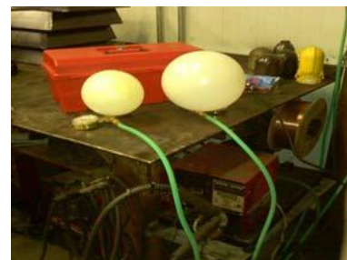
Testing flow valves Left: with valve, Right: without valve
