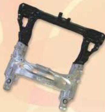
F-tech shared the “60<sup>th</sup> Okochi Memorial Technology Award” with Honda Motor Co., Ltd. and another company. It was for the hybrid subframe development technology that has the Friction Stir Welding (FSW) technology which can continuously join dissimilar metals, such as aluminum and steel. This technology is used for the Honda Accord model (North America).
