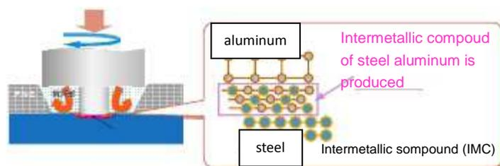
Joined by the intermetallic compound produced between the steel and aluminum
