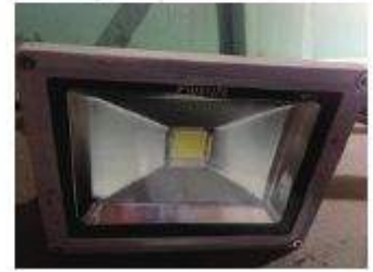
Replace the lighting lamp in the welding robot process with an LED projection lamp
