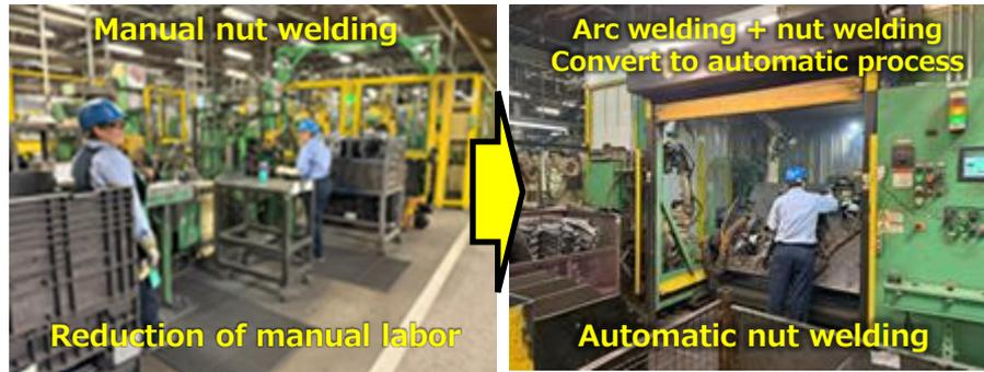
Reduced the number of staff by converting manual nut welding using a spot welder to automatic welding utilizing a transfer robot in the arc welding process.
