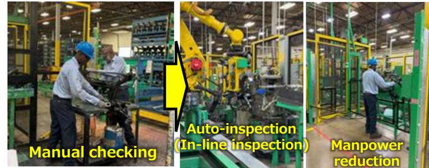
Introduced automatic inspection using QA machines to replace the manual visual inspection of all items, which allowed us to reduce manpower.
